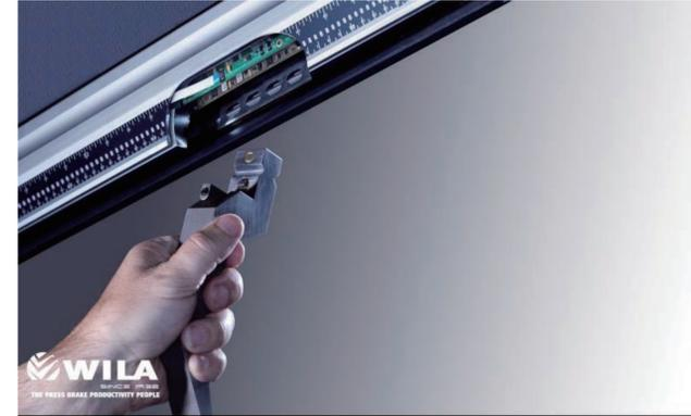
The WILA TIPS system is an integrated part of the press brake control system, and helps to identify tools and to continuously read their position. The tools are localized and identified irrespective of whether they are located in the upper clamping, lower clamping or storage system.
